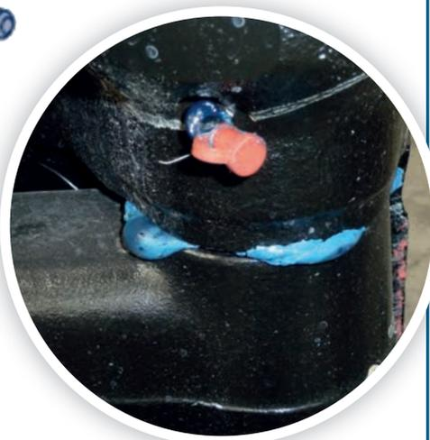
its steering pivot while the grease is applied so the cams ride over each other. The application should continue until fresh grease appears between the washers. Ideally, you'd have the trailer over a pit."
